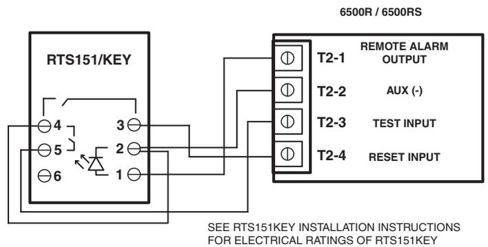
**Figure 4: RTS151KEY Wiring**
