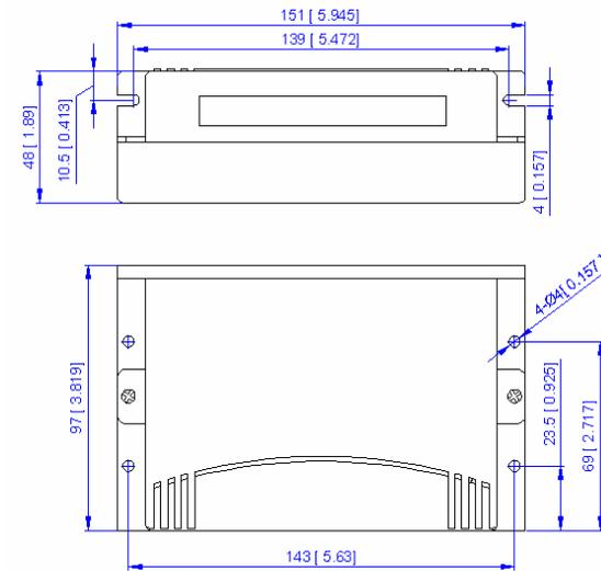
Figure 1: Mechanical specifications
