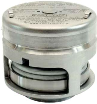
2½" BSP Super Maxi Emergency Relief Valve - 2½" BSP male connection with 65mm nominal bore. Suitable for a pressure range of between 2 - 75 PSI (0.14 - 5.17 Bar) and a vacuum range of between 0 - 26" Hg (0 - 0.88 Bar). Contact parts manufactured in 316 stainless steel. Fitted with Fortyt seals as standard. Complete with rubber/PTFE tank seal.
