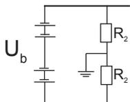
$$R_2^* = \text{Max} \frac{U_b}{2 \Delta I_{\text{set}}} \Omega$$
