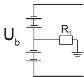
$$R_1^* = \text{Max} \frac{U_b}{4 \Delta I_{\text{set}}} \Omega$$
