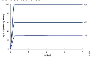
Example function: DN 40 VCL040F200 with preset max. volume flow 7500 l/h
