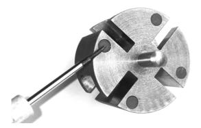
Figure 21 - Rotor with small magnets
