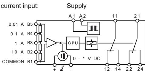
Control output and 2 relays, only in 45 mm. housing.
