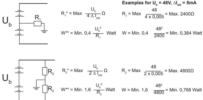
\* The calculation of the resistor is based on a safety factor of 2 corresponding to a detection of a short from one pole to ground down to half battery voltage. A resistor selected according to the maximum resistor value as calculated above will limit the leak current to 2 times  $\Delta I_{set}$  in case of direct short to ground. If it is a branched circuit with distributed "acceptable" leaks, it is recommended to use a lower value of the resistor.
