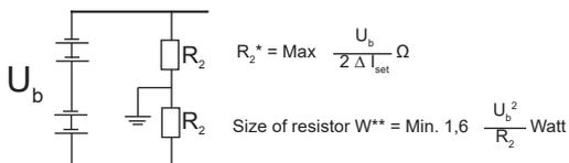
\* The calculation of the resistor is based on a safety factor of 2 corresponding to a detection of a short from one pole to ground down to half battery voltage. A resistor selected according to the maximum resistor value as calculated above will limit the leak current to 2 times  $\Delta I_{\text{set}}$  in case of direct short to ground. If it is a branched circuit with distributed "acceptable" leaks, it is recommended to use a lower value of the resistor.
