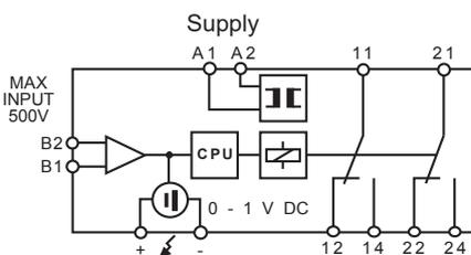
Control output and 2 relays, only in 45 mm. housing.
