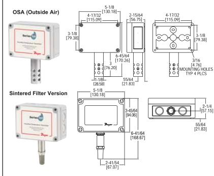
The Series RHP Humidity and Temperature Transmitter offers flexibility, high accuracy, long term stability, and reliable operation. Utilizing the duct and outside air mounting configurations, the Series RHP monitors and controls humidity or both humidity and temperature in a building energy management systems, commercial and residential HVAC applications, clean rooms, museums, and climate
