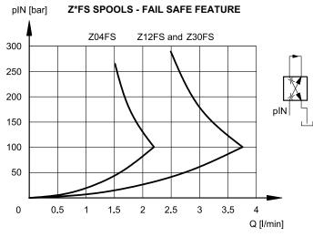
Flow  $P \rightarrow B / A \rightarrow T$  with valve in fail safe position, depending on the incoming pressure.
