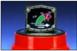
The direct mounting differential pressure gauge is fitted as standard on filters 3/4" and larger (Except AC/ACS/AX filters). Highlighting the most economical time to change the filter element.
