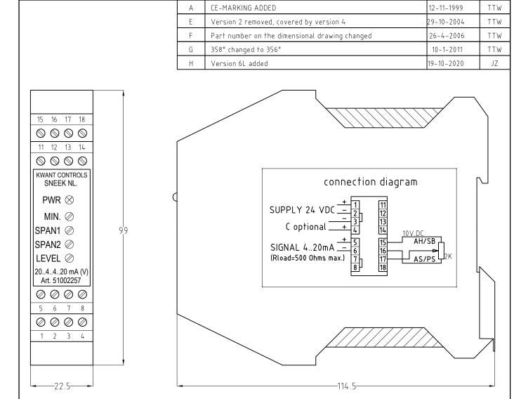
PWR = LED-lamp indicating the presence of the supplyvoltage
