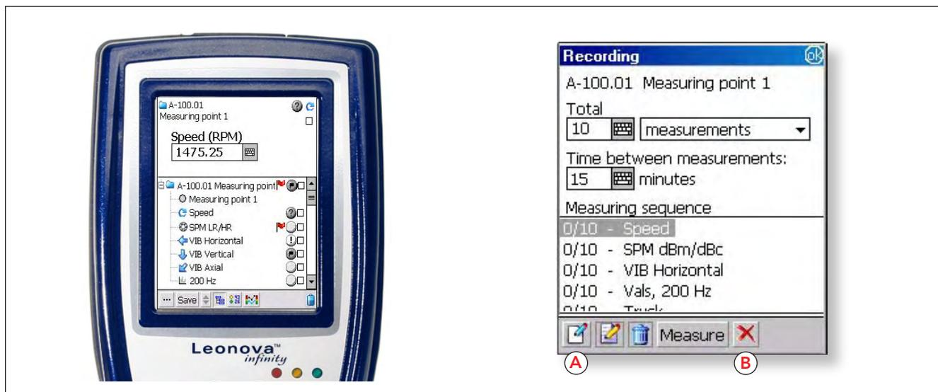
Recording is an optional Leonova function with unlimited use. It allows the user to measure simultaneously with up to three different transducers and record measuring results for as long as the battery charge will last. Thus, 'Recording' is an analysis tool that can show the interaction of various condition parameters over time.
