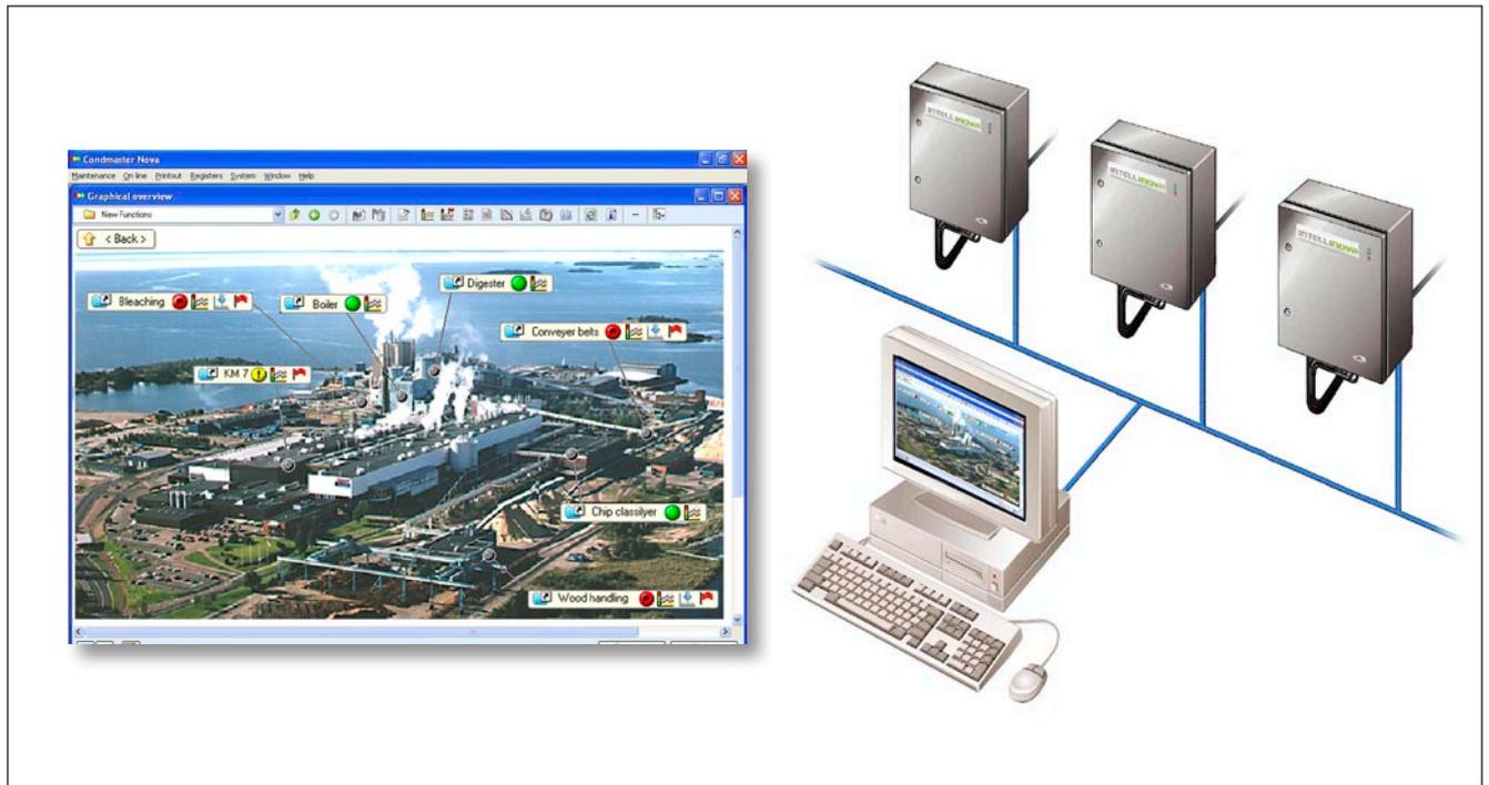
The Intellinova module in Condmaster®Nova enables the software to communicate with all Commander Units, equipped with a user selected combination of measuring units for bearing and/or vibration monitoring. Units for analog in/out are also available.
