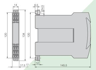
Fig. 9. SINEAX SI 815-1.... (housing **\$17**) screw hole mounting brackets pulled out.
