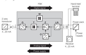
Fig. 3. Block diagram.
