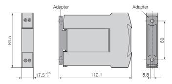
Fig. 7. SINEAX SI 815-5.... (housing **N17**) with adapter for wall mounting.
