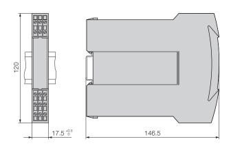
Fig. 8. SINEAX SI 815-1.... (housing  $\bf S17$ ) clipped onto a top-hat rail (35 × 7.5 or 35×15 mm, acc. to EN 50 022).
