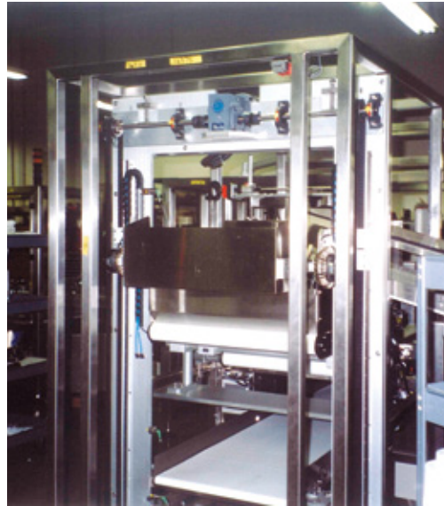
DualVee is used to raise, lower and guide product from one conveyor line to another for this pharmaceutical, cosmetic and personal care packaging machinery.
